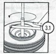
Demount the bottom bead in the same manner as above. The angle of the mongoose tool against the center post can be varied to accommodate operator height or rim depth without affecting ease of operation.
