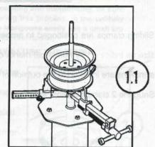
When servicing bearing-center wheels, use the center shaft that matches the bearing size of the wheel, 1/2"(12.7mm), 5/8"(15.9mm) or 3/4"(19mm). Once the wheel is positioned, insert the appropriate post into the wheel bearing.
