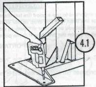
Drive 3"(76.2mm) concrete anchors into holes and tighten anchor nuts.
