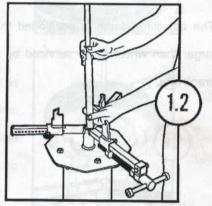
When servicing hub-center wheels the large diameter post is used. Insert post directly into center of arms, once the wheel is positioned.
