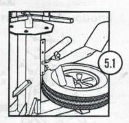
Insert demount bar into shoe and pry down to break bead. If necessary, turn tire 90 degrees and repeat the process. To break the bead on the other side, turn the wheel over and repeat this step.
