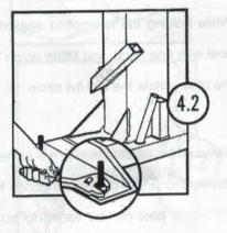
Position the Jaw Frame Weldment on top of the Main Stand Base and tighten securely using the 1/2"(12.7mm) cap-screws and nuts provided.
