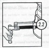
Wheel is placed in position. Wheel rim is pushed against the two sliding clamps. Insert the appropriate center post into the wheel center seating it into the center hole of the changer. Tighten the adjustable clamp to secure wheel.
